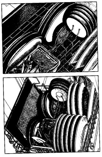
The convertible bowl tines in the right rear corner can be folded to provide either narrow or wide spacing. This allows flexible loading of a variety of articles such as serving bowls, plates, pans or casserole dishes.
